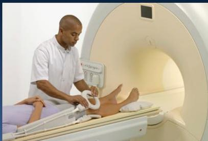
Do not create loops with coil wires
